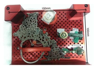
Samples are mounted and held in place with clamps and spacers. Small springs beneath the sample push the sample upwards.
